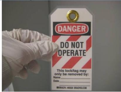
When you see blue “System in Service” sign, or a red and black “Danger: lockout-tagout sign:, do not attempt to start equipment and do not remove the signs.
