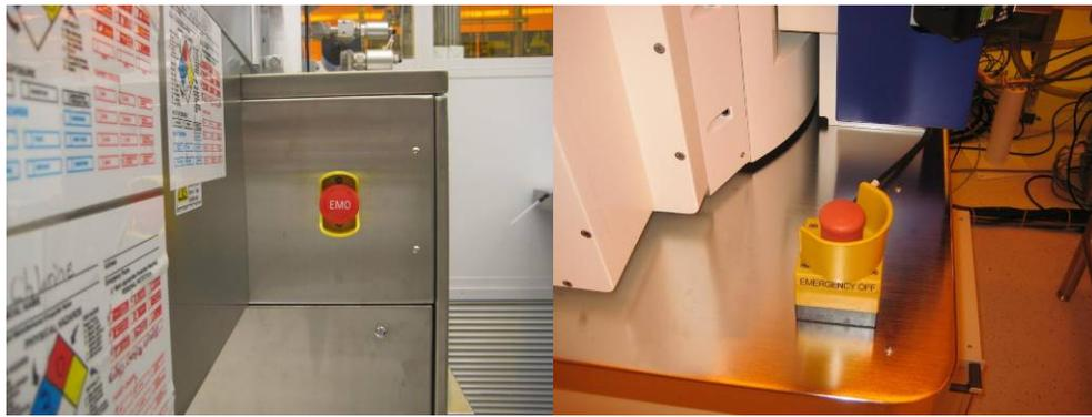
1. Use red “Emergency Machine Off” buttons to de-energize equipment during emergencies.
