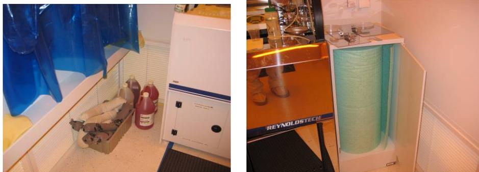
1. Spills less than one gallon inside a wet bench can be cleaned up using absorbent pads on floor near wet benches.
